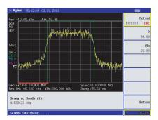
The occupied bandwidth measured in dBc.
