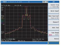
IBOC-AM measurement with N9340B IBC
