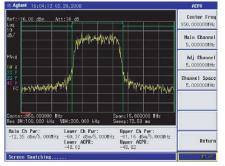
Center frequency, main channel bandwidth, adjacent channel bandwidth, and channel space can eadily be set.
