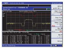
The spectrum emission mask shows the main channel power and the power level vectors relative to in-channel power for each out-of-channel frequency range.
