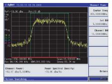
It is quick and easy to set center frequency, integration bandwidth, and channel bandwidth.
