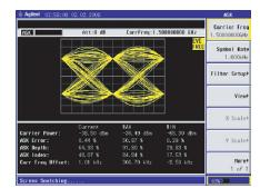
The Eye Diagram of ASK also shows the metrics with detailed parameters.
