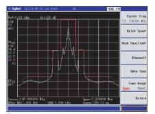
IBOC-FM measurement with N9340B IBC.
