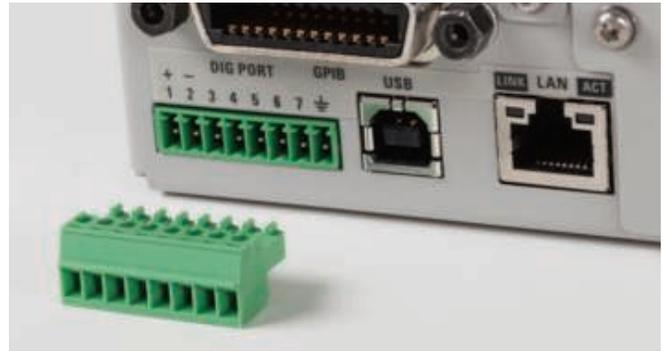
Figure 11. Digital control port on rear panel
