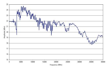
Quoted specifications between 15 and 35 °C. Maximum output power typically decreases by 0.2 dB/ °C 1. for temperatures outside this range.
