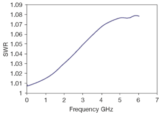
Typical SWR, 100 kHz to 6 GHz ( 25 \pm 10^\circ\text{C} ) for N8482H power sensor
