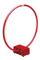
The preamplifier helps this loop antenna produce good sensitivity and almost constant antenna factors when testing for EMC applications. A preamplifier is built into the base and provides a 50-ohm output.
