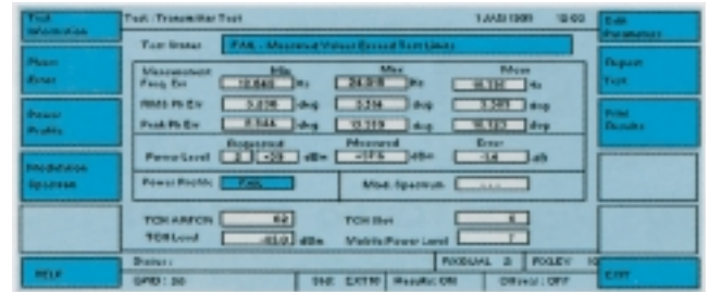
Combined transmitter test for rapid measurements of all key transmitter parameters.
